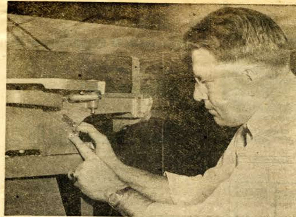
Al Anderson, tools expert, shows how | should remain as shallow as possible depth of cut index on jointer-planer | for each pass for maximum of safety.
