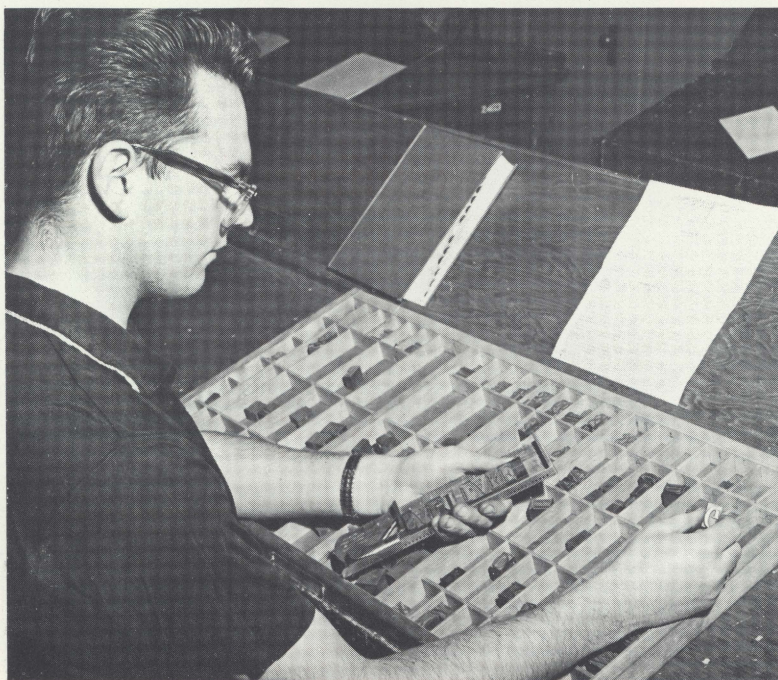
Byron Mills (Printing, '61) sets type in his "stick," a basic skill that future printers learn in classroom at Trade Tech.
